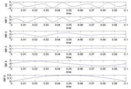
Fig 5 IMFs obtained by sifting process on sample signal
